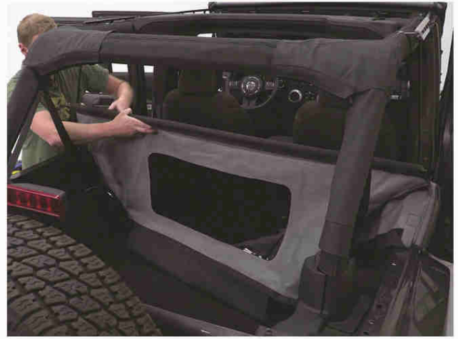
9 insert cargo bar in the pocket and position the top on the car
