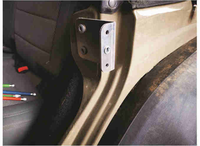
3 fix the panel brackets with OEM bolts
