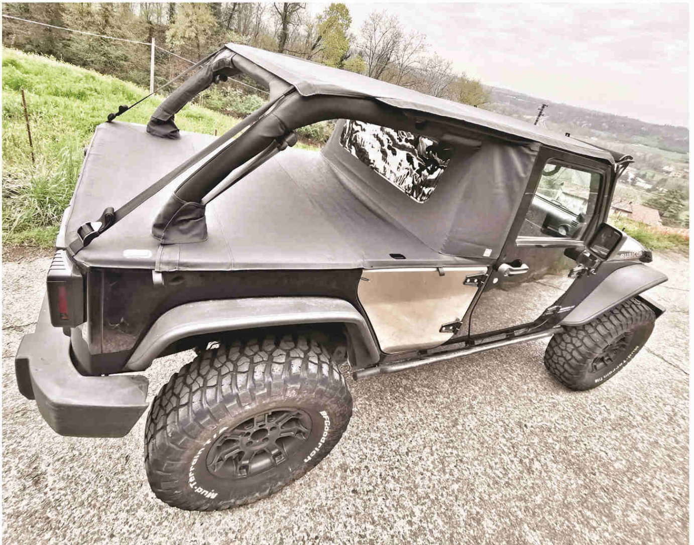
16 check all top tension for a perfect fitting
