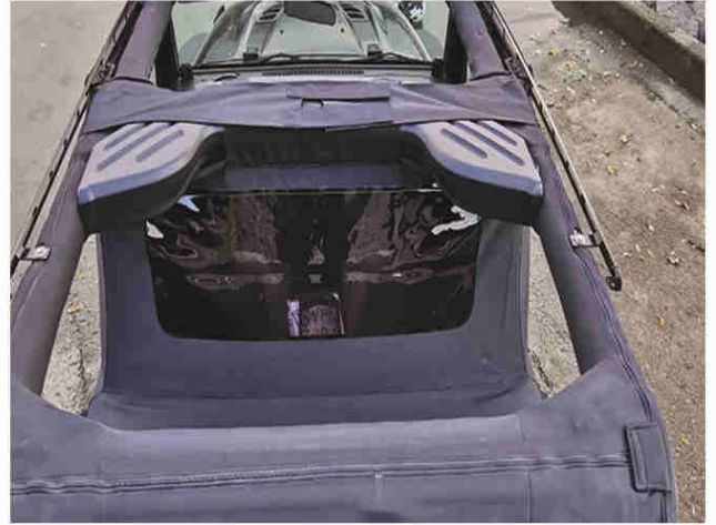
15 close upper parts over the roll cage
