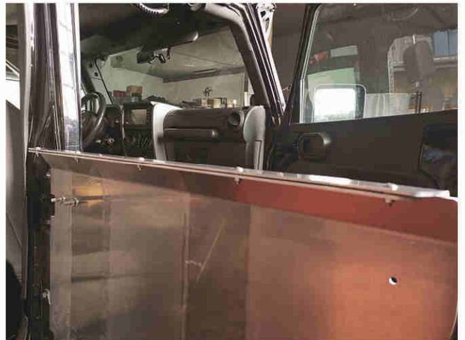
5 bolt the panel channels with M5x20
