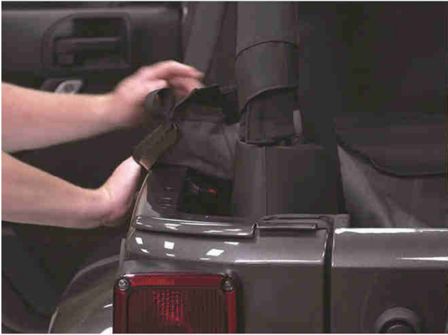
14 slide in plastic strip on the sides
