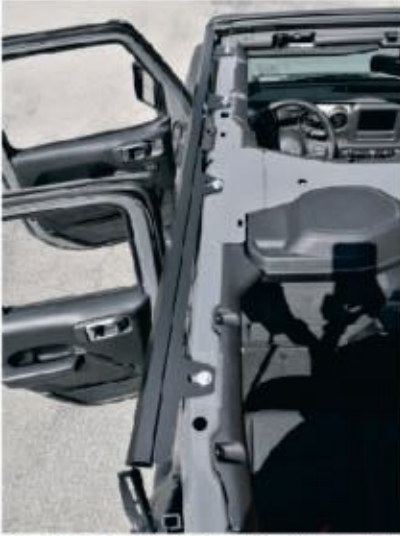
7. Bolt 2 (M8x60+2wash. + SL nut) Nut up!
