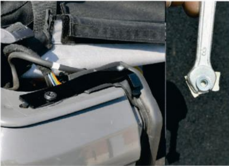
18. Fix tailgate plate (help yourself with some tape)
