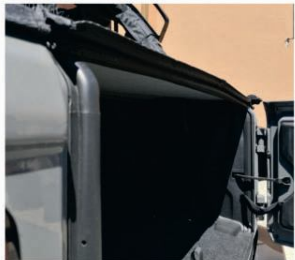
14. Place tailgate bar and fix velcro giving to the top the right tension
