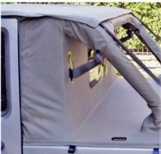
13. Insert all plastic strip with special attention to corners
