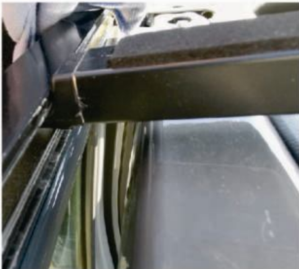
18. Fix tailgate plate (help yourself with some tape)
