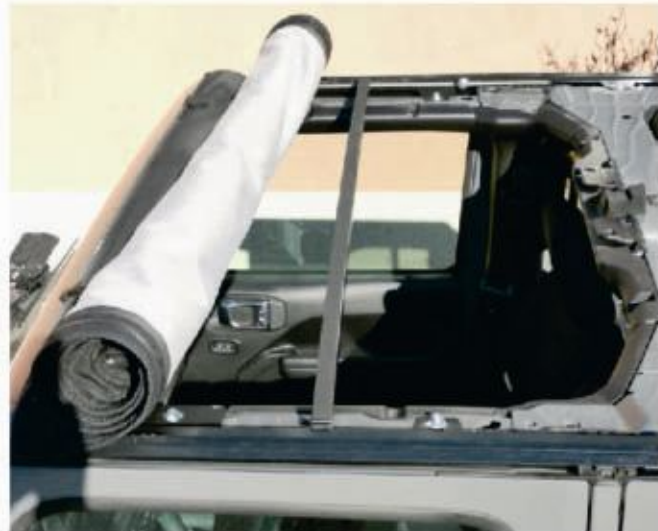
19. Position the top bar at the middle of the front space. Side inserts as in the picture.
