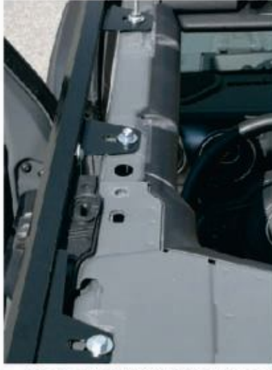
8. Bolt 3-4 (M8x75+2wash. + SL nut) Nut Down!
