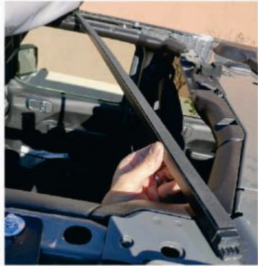
19. Position the top bar at the middle of the front space. Side inserts as in the picture.
