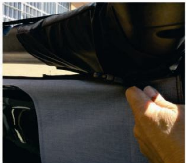
10. Pull Belt 1 from both sides keeping window centrally
