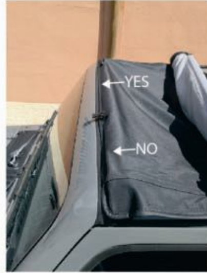
14. Release Top buckles and verify front fabric on windshield seal
