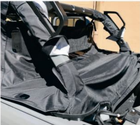
7. Temporarily fix velcro around rollcage
