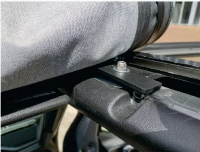
15. Tighten windshield bar nut 30Nm
