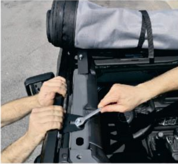
13. Tighten Bolts 2,3,4 while you pull the door channel out
