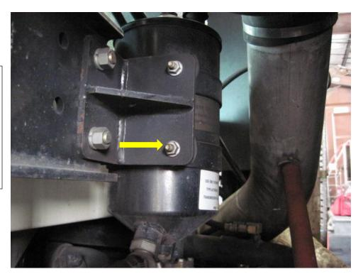
An M-181-A bracket is shown here mounted to the back side of the Eco-Pur mounting bracket. Proper orientation of the M-181-A is important to permit filter clearance once mounted. Only 2 bolts will be used to secure the brackets together.
