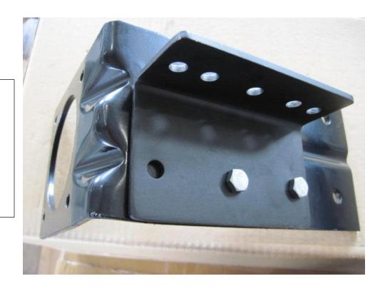
Once the Eco-Pur brackets are secured using the bolt that was removed, drill an additional hole through the existing hole in the M-181-A bracket making sure the Eco-Pur bracket is level. Secure it with one of the 5/16" bolts supplied with the installation kit.
