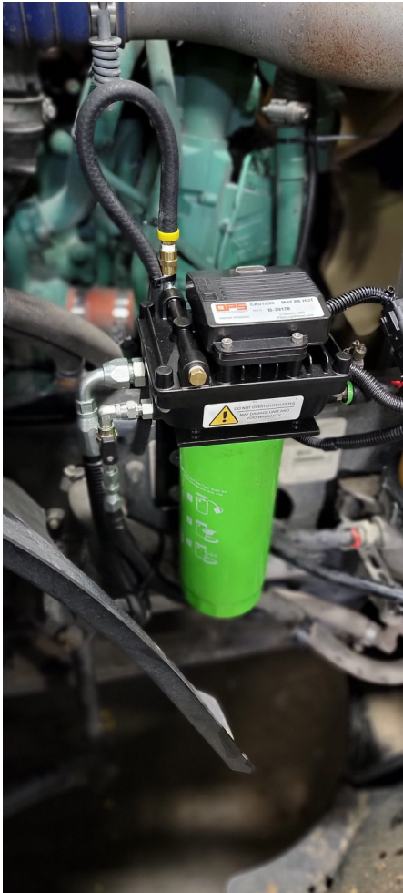
UNIT IS MOUNTED TO THE FRAME RAIL TO THE RIGHT SIDE OF THE ENGINE. FOUR HOLES WILL NEED TO BE DRILLED
