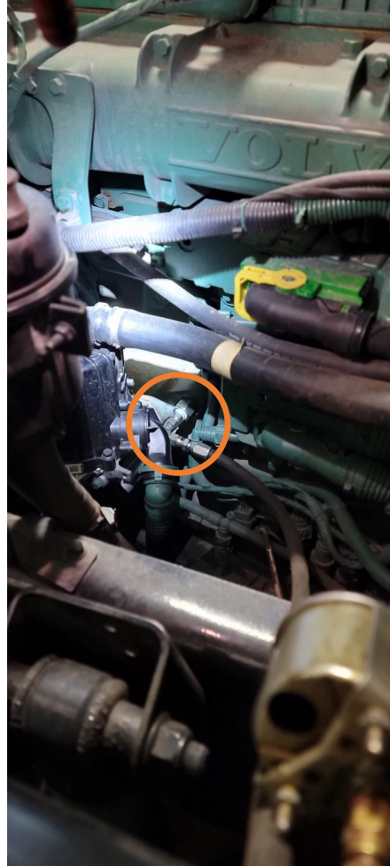
OIL FEED IS LOCATED ON THE LEFT SIDE OF THE ENGINE TO THE LEFT OF THE ECM
