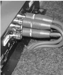
RCA cables routed through slits in the vehicle's carpet, and connected to the amplifier's signal inputs.
