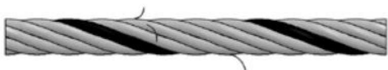
THREE WIRES BREAKS IN WITHIN ONE GROUP WITHIN ONE LAY
