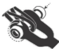
Now mount the main cable on one of the two sides to the turnbuckle (Place that is the least easy to reach.) The reason for this is that you have to tighten the cable at the other end - of course you prefer the place that is the lowest at the ground or the easiest to reach.)
