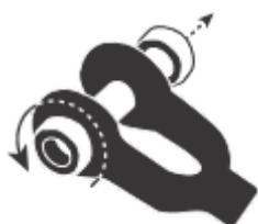
Insert the two ends of the loop in the turnbuckle jaw and secure the nuts to the bolts in the jaw.
