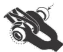
Now mount the main cable to the turnbuckle (Place that is the least easy to reach.) The reason for this is that you have to tighten the cable at the other end - of course you prefer the place that is the lowest at the ground or the easiest to reach.)
