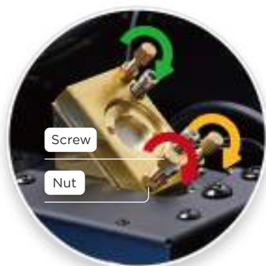
The rotation directions of mirror adjustment screws of the third reflective mirror.
