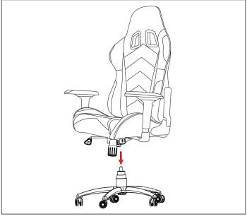
Caster wheel, Five-star base, Gas piston and Piston cover Installation Insert the gas lift piston into the five-star base and then slide the piston cover over the gas lift.
