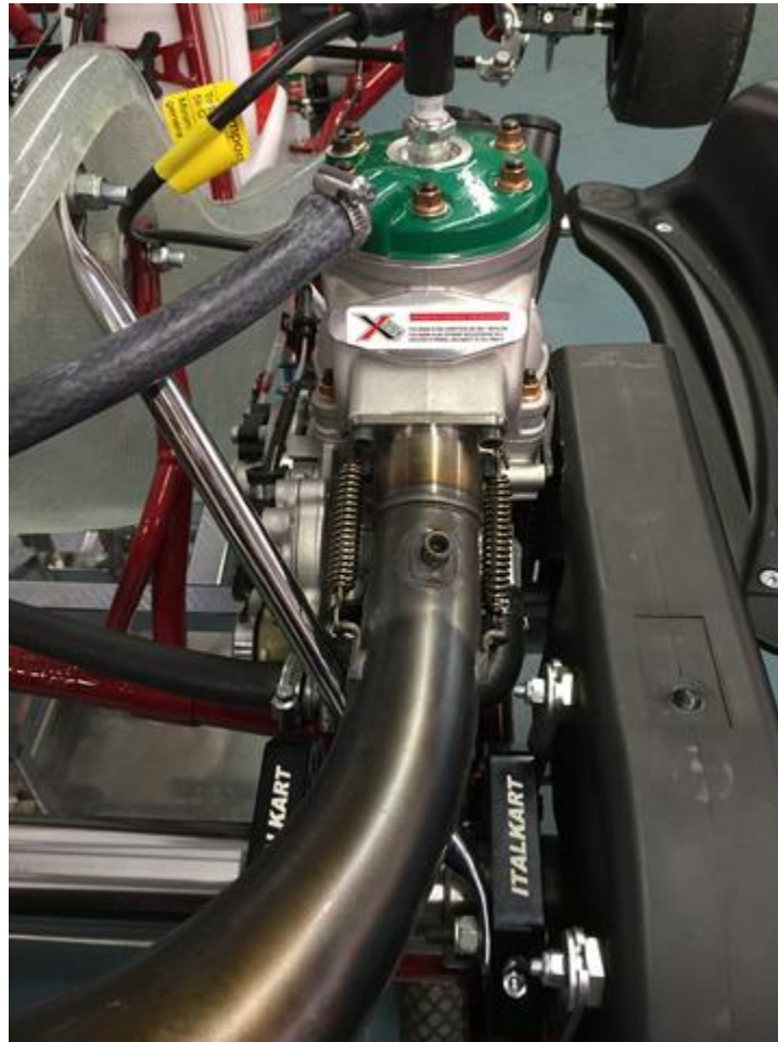
Figure 3-4 Exhaust System Placement
