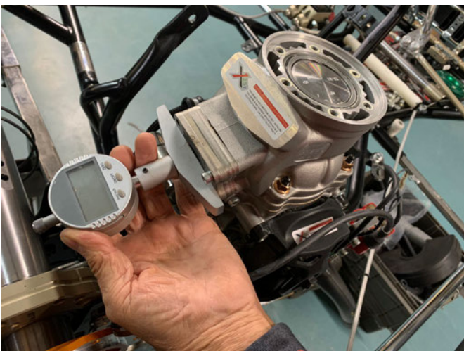
EXHAUST DUCT LENGTH CHECK
