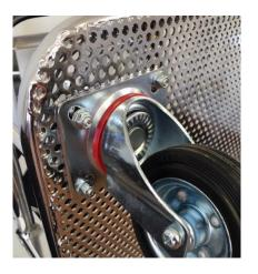
Mount the casters to the base. On the Chrome Stiletto Kart Stand, the longer bolts go through the holes in the cross brace, and the short bolts are used in the remaining holes.
