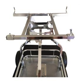
Install hooks and adjust them to the width of your kart. The hooks will latch on to your rear side pod bars, just outside the frame. NOTE: Hooks must be installed on the wider end of the top frame, above the large wheels.
