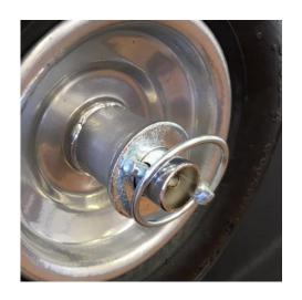
Install the wheels to the axle using the large washer and pin.
