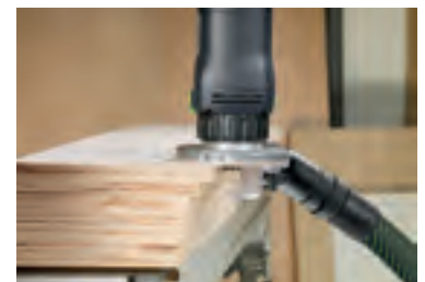
Chamfering plastic or solid wood veneer.
