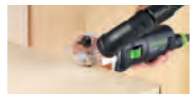
Flush trimming of plastic or solid wood veneer.
