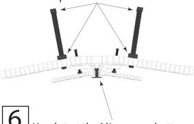
Hand start the Micro versa button into the provided hole. Tighten with 5/16" wrench until the button sits flush on the stick.
