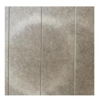
The panels are 'factory finished', meaning they are cut to size and routed, but not hand sanded before delivery. On some profiled panels (notably Shaker and Slim Shaker), very light indentations may be present in the panels from machining – these are very easily sanded out and are not considered defects. The indentations are not always visible before painting therefore sanding is a must before painting begins.
