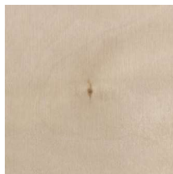
knots, pin knots black knots & intergrown knots
