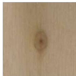
knots, pin knots black knots & intergrown knots
