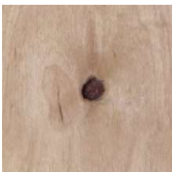
knots, pin knots black knots & intergrown knots
