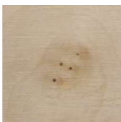
knots, pin knots black knots & intergrown knots
