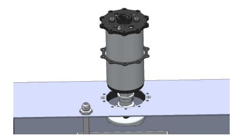
10. With the pump inserted into the tank, take the supplied socket head cap screws and washers and tighten them down. Do not over tighten as it will break or damage the washers. The finished product should look like **figure 1-8.**
