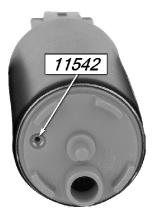
Please note the location of the vapor-purge port for your model Stealth 340, as illustrated above. During installation, be certain to check for and eliminate any blockage or restrictions to this port. Failure to do so may result in slow or no priming and may damage your 340 pump due to dry run.
