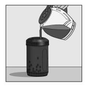
Step one: Brew fresh coffee directly onto the recessed area of the HyperChiller's lid with your compatible single cup brewer, or carefully pour it in with a carafe. Liquid will flow through the opening at the bottom of the lid, and into the cooling chamber.
