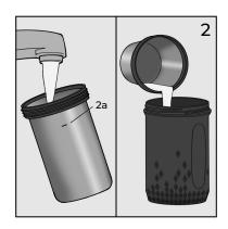
Fill large stainless steel cup with water up to the indented mark (2a), and empty contents into the black HyperChiller cup.
