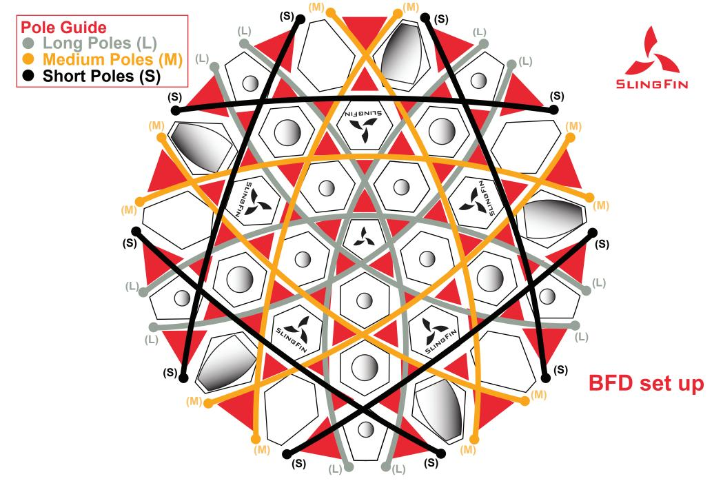
Assemble the 5 Silver and Black poles (S) and install the pole ends into grommet straps marked (S).
