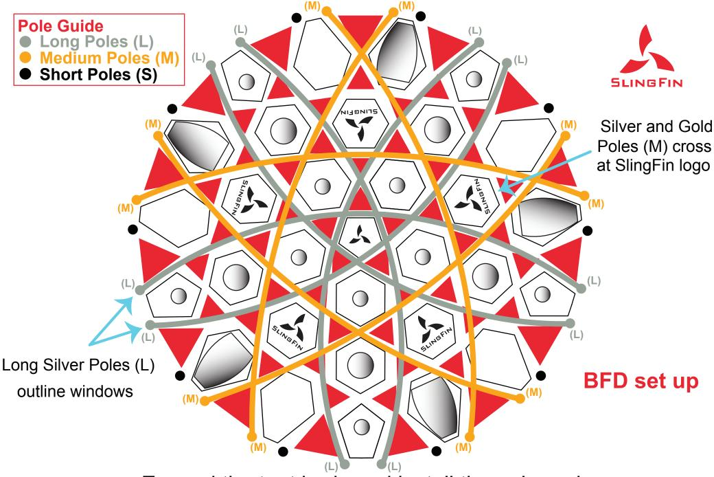
Expand the tent body and install the pole ends: Long Silver Poles into grommet straps marked (L) and Silver and Gold Poles into grommet straps marked (M).
