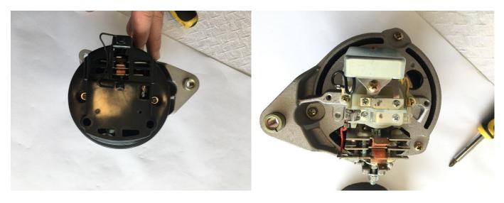
Once screws are removed from front plate, rotate front plate until opposite mounting point lines up with rear mount.
