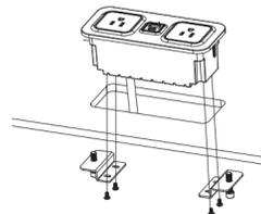
3. Secure CubieMod to the desk by tightening the 2 allen bolts.
