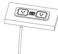
4. Plug directly into wall AC outlet. Do not plug into another surge protector or extension cord.
