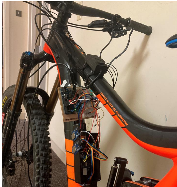
(Figure 21, Installed Arduinos and MPU 6050s)
