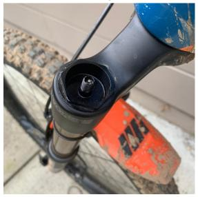
Step 3: Install the fork tracer, tighten the MI supplied air cap until it's almost tight, but allows movement of the Flexure Arm.
