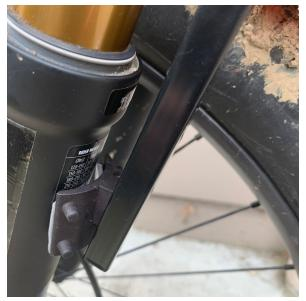
Step 6: Before you stick the Wiper to the lower fork, make sure the magnet is at least 5mm into the position sensor membrane.
