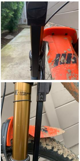
Step 9: Connect to the Fork Tracer with MotionIQ, connect to the fork, choose your bike (specific bike model or generic hardtail, if hardtail you will have to set the fork travel length). Then calibrate. This will ensure that the Tracer is mounted correctly. If you get a calibration error, ensure that your Wiper is mounted so that the sensor travel is slightly longer than the fork travel.
