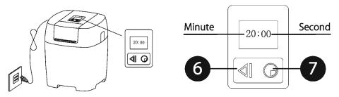
6. Each time the Reset button is pressed, the running time is added one minute with a "beep" in sequence:
