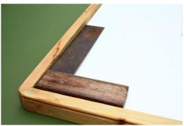
Your jig must be 100% level as any unevenness will affect the quality of the build and may make the latter stages of construction impossible (this is down to the fine tolerances the components are machined to).
