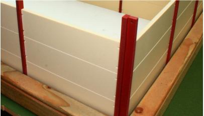
Once happy with the above, run a thin line of glue down the RSJ of the back wall and offer up the side wall. Leave in place for 5 minutes before proceeding to the next stage.
