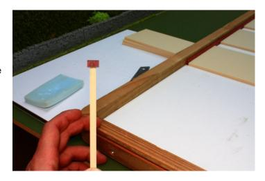
Place an RSJ upright into the corner of your jig in an upright position, then apply a small amount of glue to both edges of your wall section, offer the 2 parts up and quickly offer up the second RSJ, making sure the walls are central to the RSJ.
