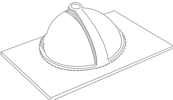
5. Attach the sink clips by placing the long end of the bracket flat against the sink lip. Screw the wing bolts through the brackets and bolt holes and tighten snugly.
