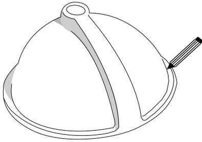
3. Remove the sink from the vanity top. Apply a generous bead of silicone around the sink rim.
