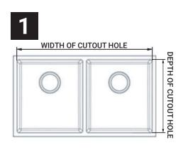
Measure the internal width and depth of the sink, cut out the bench top at desired location.
