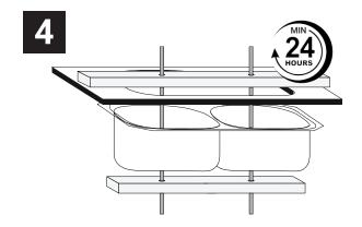
Lay a timber piece across the bench top and under the sink. Place a clamp through to hold the sink in place. Leave this for **a minimum of 24 hours** for the silicone sealant to cure.
