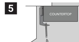
Position the bottom of the mounting clip so that it is gripping the countertop. Use a screwdriver to tighten the screws until the mounting clip is snug against the countertop.
