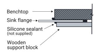
**Sandwich Technique** - Fix support board and ensure sink flange sits firmly and flat against the top benchtop surface.
