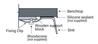
**Fixing Clips** - For solid benchtops, ensure to fix wooden blocks to the underside of the bench. One fixing clip end should rest on the wooden block and opposite end is to rest under the sink rim.
