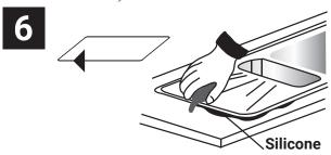
Apply weight to the top surface evenly to aid the drying of the applied silicone ensuring sink rim is evenly spaced around the cut-out. Wipe off any excess silicone.
