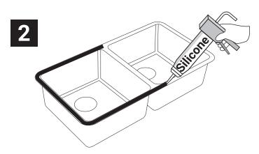
Apply silicone to the top of the sink rim. Do not let the silicone dry before the sink is fitted to the benchtop. Place sink into position.
