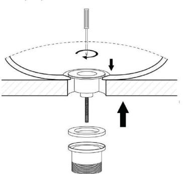
4. Re-fit plug and grate into top base. Connect pipe work and test plug mechanism by pressing plug down with running water
