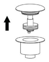
2. Fit foam washer to top base and drop fixing bolt into base
