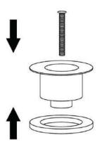
3. Place the lower base with silicon washer underneath the basin and tighten fixing bolt with phillips head screw driver
