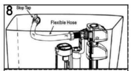
8.IF STEP 8 IS COMPLETED, SKIP THIS STEP. Fit off stop tap then connect rear water inlet valve to stop tap. Fill cistern and ensure correct water level.
