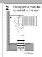
2.Lubricate the fins of the pan bend and position into waste pipe.
