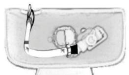
Make sure inlet valve flow are free from side of cistern wall.
