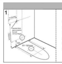
1.Rough in position of water inlet, waste outlet.
