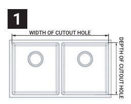
Measure the internal width and depth of the sink, cut out the bench top at desired location.
