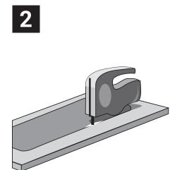
Use a proper device when cutting on the countertop. Cut according to marked cut-line.
