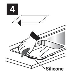
Apply weight to the top surface evenly to aid the drying of the applied silicone ensuring sink rim is evenly spaced around the cut-out. Wipe off any excess silicone.
