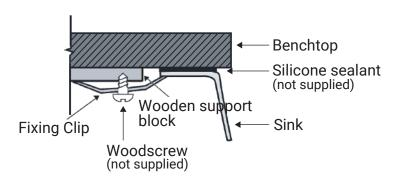
**Sandwich Technique** - Fix support board and ensure sink flange sits firmly and flat against the top benchtop surface.
