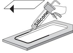
Apply a bead of silicone adhesive to the bottom of the sink rim and lower the sink into the cut-out hole.
