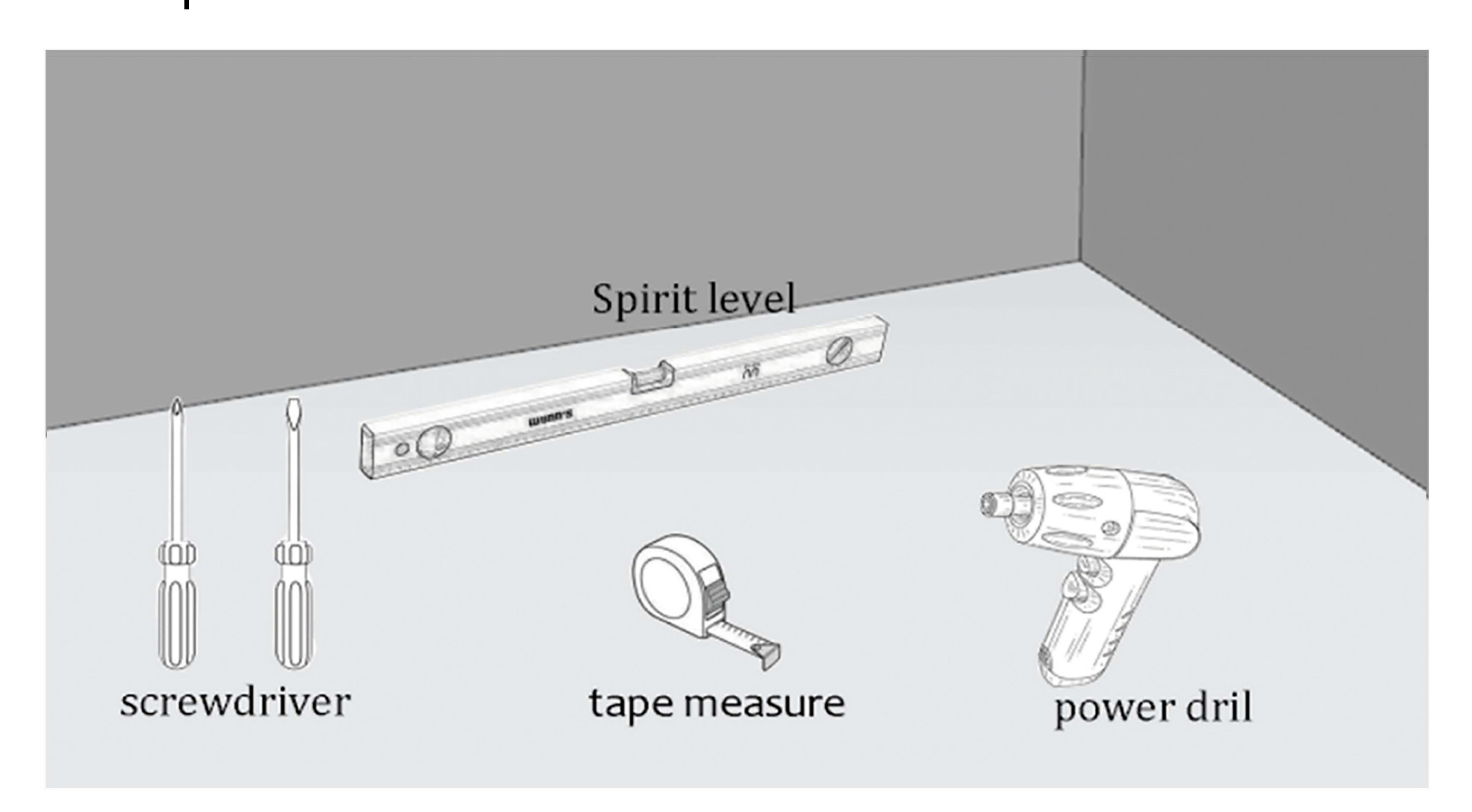
3. Confirm the installation position, use a spirit level to confirm whether the installation holes are at the same level, and then use an power drill to make holes on the wall.
