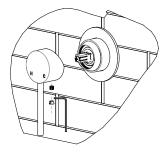
6. Fit handle on, taking care that it is pushed fully onto the cartridge stem, then tighten grub screw. Fit the indicator plug in. Taking care not to damage the decorative finish.
