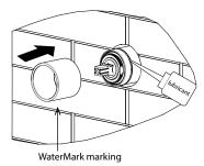
3.Ensure the surface of the mixer body is clean, apply lubricant on the O-ring, then slide trim sleeve (with WaterMark underneath) over mixer body and push it in.
