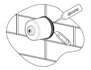
1. Seal the wall penetration between the body kit and the lining board and tiles in accordance with AS:3740 & then cut off any fitting sleeve extending out of the wall/ tile face.
