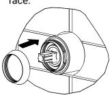
4. Screw cap onto the thread of nut and hand tighten to secure the trim sleeve.
