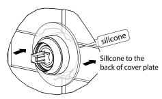
5. Apply suitable sealant to the back edge of the cover plate and push the cover plate firmly against the wall/ tile face. Wipe off excess sealant.
