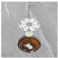
(a) Remove the circular metal cover with the level indicator from the in-floor box by removing the 4 hex bolts.
