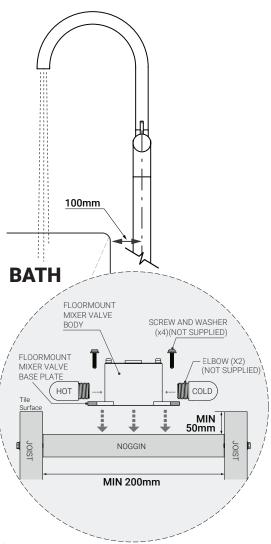
(a) First, prepare a suitable recess on the floor where you will install the in-floor box. This must have accessible hot and cold water supply inputs.
