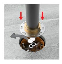
**(c)** Remove the plastic centre protective disc .Insert the hot and cold inlet pipes securely into the outlet ports of the in-floor box. Check for any leaks.
