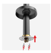
**(b)** Bolt the circular metal cover from the in-floor box to the underside of the brass threaded collar at the base of the mixer tube using supplied hex bolts.
