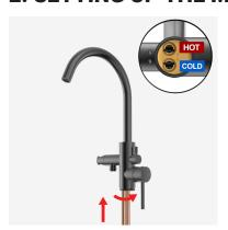
(a) Connect the hot and cold water supply pipes securely into the inlets on the base of the mixer head with correct Hot and Cold Direction.
