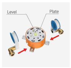
**(b)** Check the position of the outlet ports, as this is where you will later insert the mixer's inlet pipe. **Please determine the spout direction before installation. The spout direction is aligned with hot water(H).** Apply teflon or sealant onto fittings and install.
