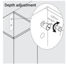
6. The gap adjustment screws are behind top white plastic covers. Remove the plastic covers inside the cabinet and turn the top screws clockwise/counter clockwise to achieve ideal gap between the cabinet and wall
