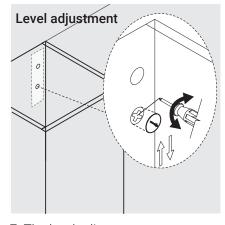
7. The level adjustment screws are behind bottom white plastic covers. Remove the plastic covers inside the cabinet and turn the bottom screws clockwise/counter clockwise to tune the height of tallboy.
