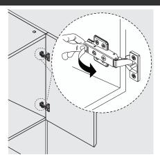
1. Remove doors. Apply finger pressure to clip at the end of hinge and pull forward to release.
