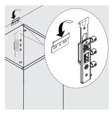
5. Hang the cabinet on and ensure the 2 brackets are fully engaged.
