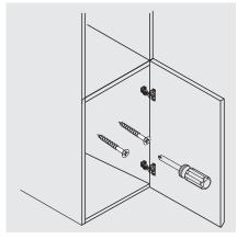
9. Once you are happy with the position of the cabinet, add extra screws to secure the cabinet to studs/ support beam.
