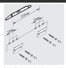
3.Install mounting bracket assembly to the horizontal beam. Ensure the brackets assembly are level.
