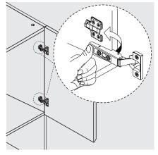
8. Put doors back to cabinet. Engage hinge arm to mounting bracket, press the back of hinge into place. When you hear a 'click' sound, the hinge is engaged.
