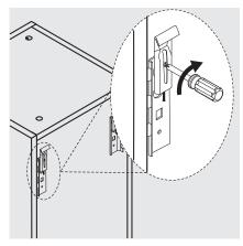
4. Locate hanging brackets in the back of the cabinet. Turn the screw clockwise so the hook will come out of side panel.
