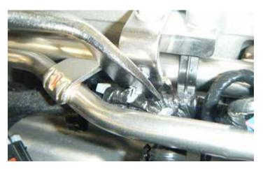
27. Using a fork type pry tool, carefully pry the wiring harness fastener clip located on the front of the passenger side fuel rail.
