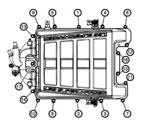
37. Seventeen (17) 10 mm head bolts secure the supercharger cover to the supercharger assembly.
