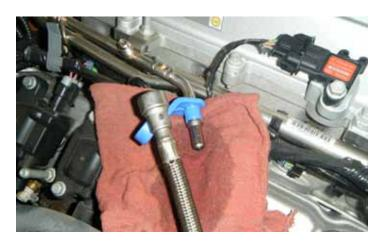
45. On the driver side of the engine, remove the lock and disconnect the fuel feed-to-rail hose from the fuel rail using the J-37088-A fuel line disconnect tool or similar tool (available from LPE, part # MAG69-12-57-001). Use a rag to catch any excess fuel that may spill from the lines.
