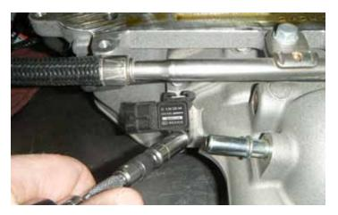
92. Connect the engine inlet air pressure sensor electrical harness.
