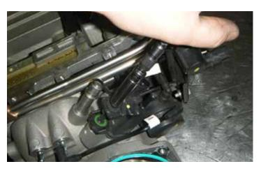
56. Using a 10 mm socket, remove the bolt to the purge solenoid from the supercharger front cover.
