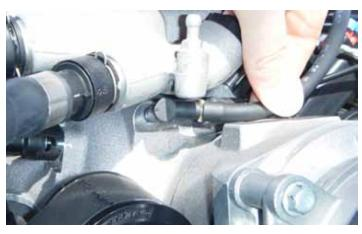
114. Connect the active exhaust vacuum hose to the supercharger front cover.
