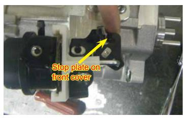
74. Hold the bypass stop plate back so that the bypass valve blade is in the closed position. The stop plate should not be touching the set screw on the bypass actuator. The set screw can be adjusted using a 3/32" Allen wrench.
