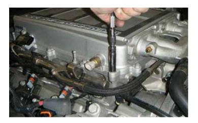
95. Install the seventeen (17) supercharger cover bolts and the supercharger cover.
