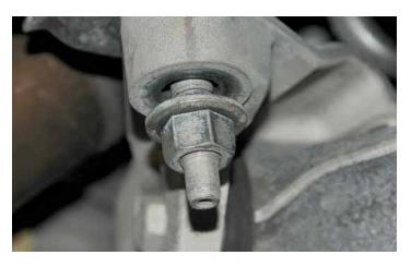
35. Loosen the engine cradle nuts such that you have roughly a 1 inch (25 mm) gap between the nut and the subframe. You should still have several turns of engagement on the threads on each nut. Do not remove the nuts from the studs.
