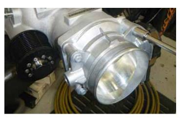
80. Install the throttle body on the supercharger front cover. Using a 10 mm socket, torque the four (4) bolts to 10 Nm (89 lb-in).
