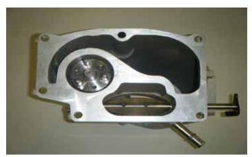
66. Apply a thin film of the supplied Permatex Ultra Black Gasket Maker to the Lingenfelter LS9 cover flange surface.
