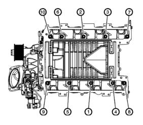
47. Ten (10) 8 mm socket head bolts retain the supercharger assembly.
