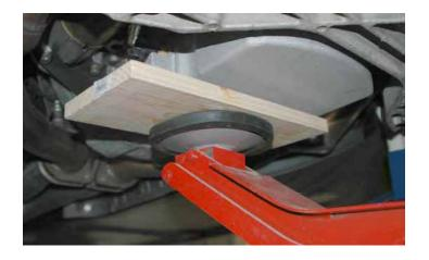
99. Using the jack raise the engine back up into position.
