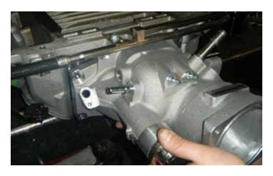
67. Install the new cover onto the supercharger assembly. The three pins sticking out of the supercharger drive shaft in the front cover go into the three holes in the plastic coupler that are not occupied by the pins from the supercharger assembly.
