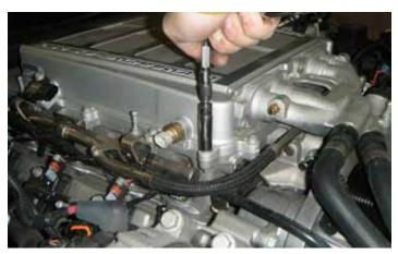
36. Starting with the back 6 bolts, remove the 10 mm bolts on the supercharger cover with a socket and extension.
