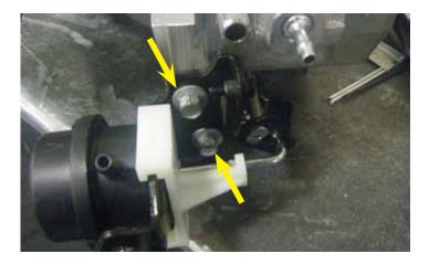
75. Install the two (2) 10 mm bolts and torque them to 21 lb-ft (28.5 Nm).
