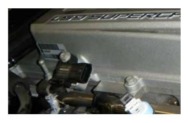
109. Connect the barometric pressure sensor electrical connector.
