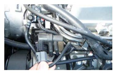
115. Connect the electrical connector to the supercharger boost control solenoid and connect evap hose to solenoid.
