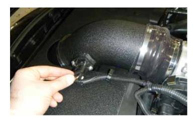
121. Connect the mass air flow sensor connector.
