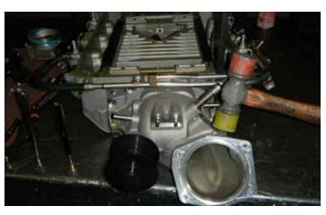
60. Using a mallet (or prybar) gently knock the front cover loose from the supercharger assembly. It is located in place by two dowels and the pins in the supercharger shaft coupler so you are just using the mallet to loosen the adhesive between the cover flange and the supercharger housing.
