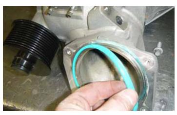
58. Carefully remove the throttle body gasket from the front cover assembly. Inspect the gasket. If it is in good condition it will be re-used later on. If it is damaged you will need to obtain a replacement gasket [GM PART #12576549].
