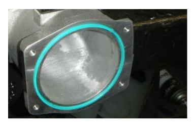
69. Install the throttle body gasket that you removed from the stock front cover onto the new supercharger front cover.
