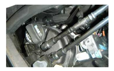
105. Connect the PCV fresh air hose assembly to the left and right valve covers and the dry sump tank.
