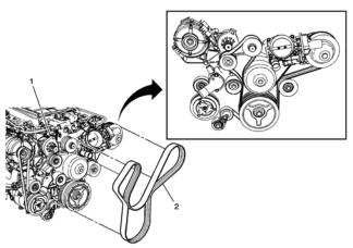
118. Install the supercharger drive belt.
