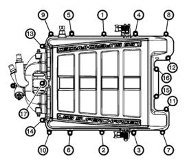
96. Tighten the bolts a first pass in sequence to 5 Nm (44 lb-in).
