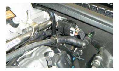
111. Connect the fuel injector and ignition coil harness connector on the driver side.
