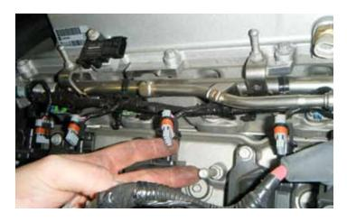
29. Disconnect the ignition coil electrical connectors from the ignition coils on the right side of the engine.
