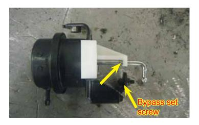
73. Use the set tool to set the actuator position [tool part # ETN86063]. Place the actuator set tool so that the actuator arm teeth are located in the position shown. Note the bypass set screw position.
