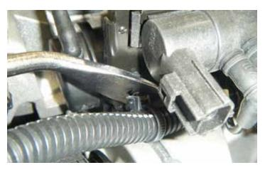
24. Using a fork type pry tool, carefully pry the wiring harness fastener clip below supercharger boost control solenoid.
