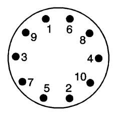
71. Apply a small amount of Loctite Blue to the supplied M4x0.7x12 socket head cap screws and, using a 3 mm Allen wrench or socket, secure the pulley to the hub with these screws. Use the pattern to the left to tighten the screws. Torque to 2.3 Nm (20.7 lb-in). For instructions on supercharger pulley removal, refer to page 34.
