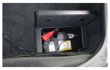
2. Open the rear hatch and open the battery compartment cover. Using a 10 mm socket wrench, disconnect the negative (-) battery cable from the terminal on the battery. Cover the cable end with electrical tape so accidental connection to the battery does not occur.
