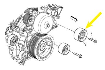
82. The idler to be replaced is the factory 90 mm idler found on the driver side of the vehicle (not the 76 mm idler found near the water pump and tensioner).
