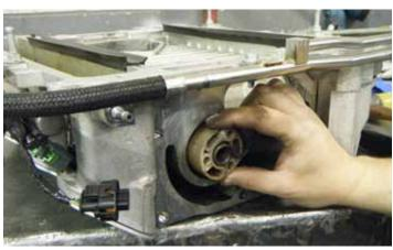
62. Remove the spring loaded isolator coupling from the supercharger assembly (or it may be on the front cover assembly).
