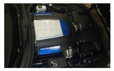
127. Start the engine and check from proper belt alignment and listen to make sure you do not have any vacuum leaks.
