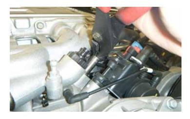
113. Connect the brake boost vacuum line to the supercharger front cover.
