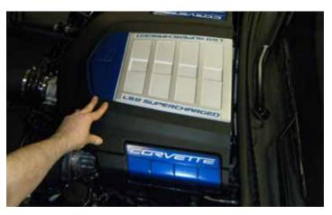
122. Re-install the engine sight shield (engine cover) by pushing down on the cover to secure it to the mounting posts.
