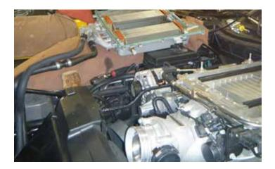
87. With the help of an assistant, place the supercharger assembly back in place on the engine. Align the dowel pin at the right front of the supercharger to the cylinder head.
