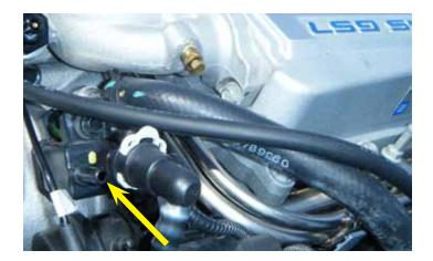
31. Disconnect the purge line from the purge solenoid on the left side of the supercharger front cover.
