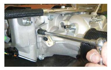
59. Using a 10 mm socket and extension, remove the six (6) bolts that secure the front cover to the supercharger assembly.
