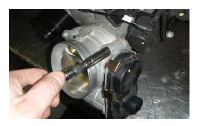
53. Using a 10 mm socket, remove the four (4) bolts that secure the throttle body to the supercharger assembly. Remove the throttle body.
