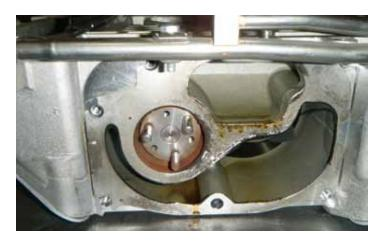
61. Remove the front cover from the supercharger assembly.
