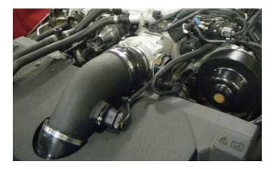
119. Install the air intake system.
