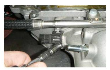
79. Install the inlet air pressure sensor onto the front cover. Using a 10 mm socket, torque the fastener to 10 Nm (89 lb-in). Plug connector back into inlet air pressure sensor.
