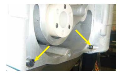
65. Remove the old dowel sleeves from the front cover/housing. Install the supplied dowel sleeves into the LS9 supercharger housing. Install the sleeves in the bottom left and bottom right hand corner of the supercharger housing. DO NOT install sleeves on the front cover.
