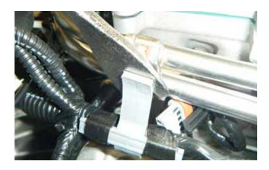
25. Using a fork type pry tool, carefully pry the wiring harness fastener clip on the front of the driver's side fuel rail.
