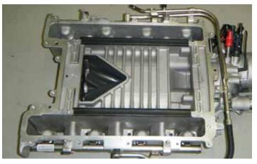
48. With the help of an assistant, remove the supercharger assembly. The supercharger, throttle body, fuel injection rail and fuel injectors may be removed as an assembly. Use care not to reposition or bend the intercooler cover dowel pins. Do not lift the supercharger assembly from the black plastic vacuum actuator as you risk damaging the actuator.
