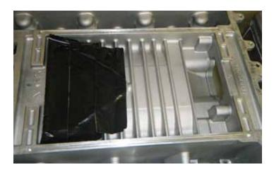
49. Cover the inlet area of the supercharger to prevent dirt or debris contamination onto the rotors.
