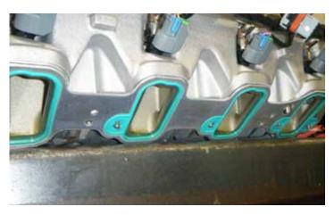
52. Inspect the intake manifold gaskets on the supercharger assembly. If they are damaged you will need to drill out the gasket rivets and install new gaskets and gasket rivets [GM PART # 19180613].
