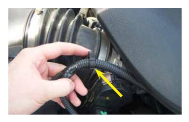
5. Remove the plastic loom holder from the factory intake duct but leave the MAF sensor harness loom in the holder. Be careful not to damage the factory plastic fastener.
