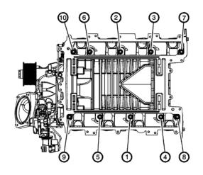
89. Tighten the bolts a first pass in sequence to 5 Nm (44 lb-in).
