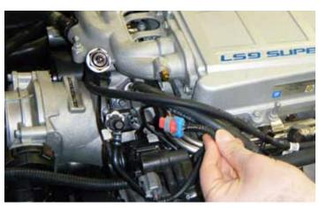
116. Connect the electrical connector to the EVAP purge solenoid.
