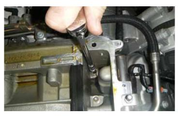
88. Torque down the ten (10) supercharger bolts, refer to the next step for the torque pattern and specifications.
