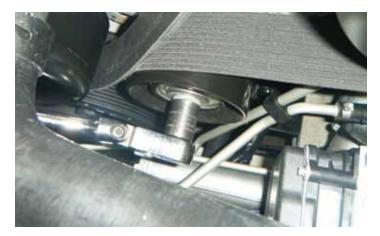
83. Using a 15 mm socket, remove the bolt that secures the factory 90 mm idler.
