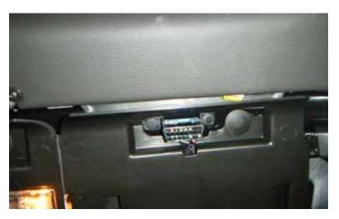
126. Install the supplied diagnostic port (DLC port) cover onto the DLC port in the driver foot well. Secure the strap that retains the DLC cover to the vehicle.
