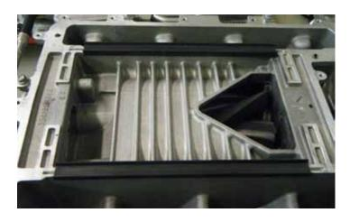
93. Install insulator seals on the supercharger assembly.
