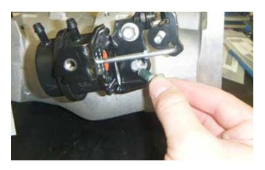
72. Using a 10 mm socket, torque the two (2) bypass actuator bolts to 18 lb-ft (25 Nm). In the new casting the bottom bolt hole is machined all the way through to the inside of the front cover so the bolt going into this hole needs thread sealant applied to the threads [Loctite 567 thread sealant or equivalent].
