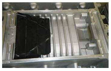
90. Remove the tape or other covering material from the supercharger housing.
