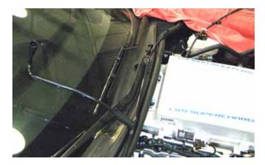
23. Move the PCV air house assembly out of the way by rotating it up and over.
