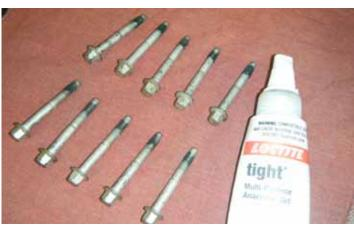
86. Apply a 5 mm (0.2 inch) band of threadlocker (Loctite Blue, GM PN 12345382 or equivalent) to the threads of the 10 supercharger bolts. Place the ten bolts into the supercharger.
