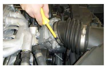
10. Using a 5/16" nut driver or socket, loosen the clamp on the throttle body
