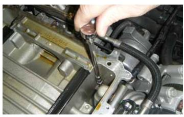
46. Using a 8 mm socket and extension, remove the supercharger bolts.
