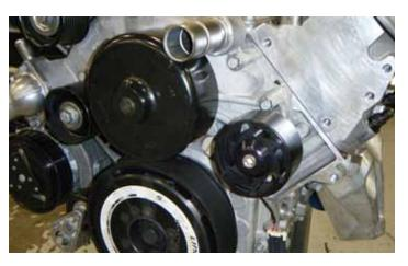
84. Place the supplied idler locating spacer on the back side of the idler. Place the supplied dust shield/cover on the front of the idler pulley. Put the supplied bolt through the idler and install the assembly on the engine.
