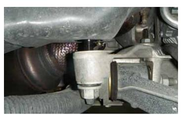
100. Using a 21 mm socket, tighten the four engine cradle stud nuts (two on each side) and torque to 110 Nm (81 lb-ft). You can now remove the jack from under the engine.
