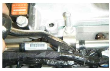
26. Using a fork type pry tool, carefully pry the wiring harness fastener clip located on the rear of the driver's side fuel rail.
