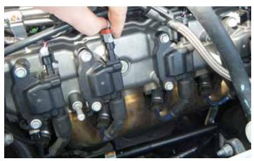
30. Disconnect the ignition coil electrical connectors from the ignition coils on the left side of the engine.
