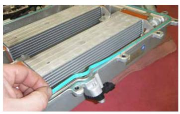
94. If you removed or are replacing the supercharger cover seal, install the supercharger cover seal.
