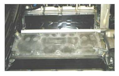
85. Make sure the cylinder head and engine area are free of loose debris. Remove the tape from the cylinder head intake ports.
