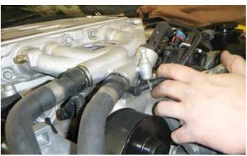
14. Disconnect the active exhaust vacuum hose that routes from the left side of the engine compartment to the front of the supercharger.
