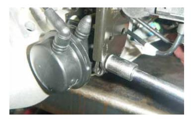
77. Install the boost control solenoid bracket assembly onto the front cover. Using a 10 mm socket, torque the fastener to 10 Nm (89 lb-in). Replace all vacuum hoses.
