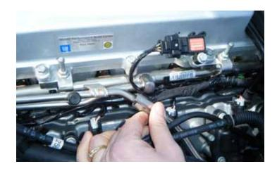
97. Reconnect the fuel line and safety clip on the passenger side of the vehicle.
