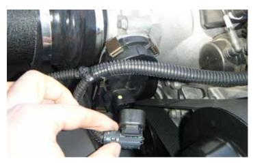
120. Connect the throttle actuator electrical connector.
