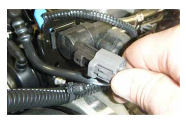
13. Disconnect the electrical connector from the supercharger actuator solenoid at the left front of the supercharger.
