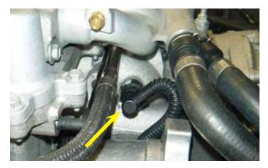
91. Connect the PCV dirty air hose line to the passenger side of the supercharger front cover.
