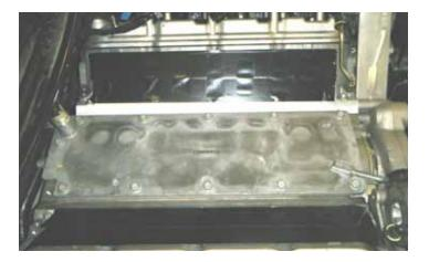
51. Cover the intake ports on the engine with tape or rags to make sure nothing enters the engine.
