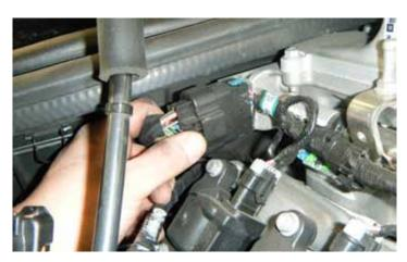
112. Connect the fuel injector and ignition coil harness connector on the passenger side.
