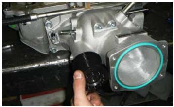
70. Install the supercharger pulley onto the hub on the supercharger shaft.
