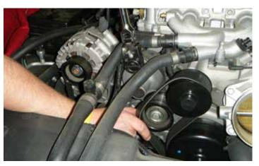
12. Remove the supercharger drive belt by using a 1/2" breaker bar to rotate the supercharger belt tensioner and then remove the supercharger belt from the pulleys and tensioner.
