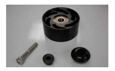
81. If you are using a pulley combination that requires a different idler, replace the factory idler at this time. Follow steps 79 to 81 for installing the new idler. See table 1 on page 37 for information on what size idler is needed for different pulley combinations.
