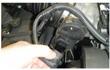
6. Disconnect the throttle actuator electrical connector from the throttle body.
