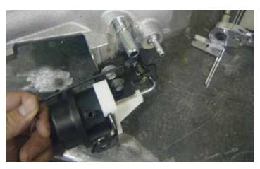
76. Tighten the set screw so that it barely touches the stop plate on the front cover. After the initial contact, tighten the set screw 1/8 to 1/4 turn *more* to set the bypass valve blade into position. The set screw should now be touching the stop plate on the front cover. This will prevent the bypass valve blade from getting stuck on the front cover casting. Remove the bypass actuator set tool.
