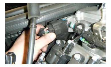
19. Disconnect the fuel injector and ignition coil harness connector from the passenger side of the engine.
