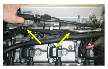
107. Re-attach the two (2) wiring harness fastener clips on the passenger side of the vehicle.
