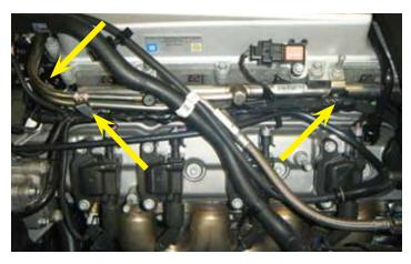
106. Re-attach the three (3) wiring harness fastener clips on the driver side of the vehicle.
