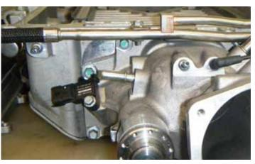
68. Install the six (6) cover bolts with a 10 mm socket and extension. Torque to 27 Nm (20 lb ft). The torque sequence is not critical on this component. With the plastic cover removed from the end of the shaft, tap the end of the shaft with a rubber mallet to seat the plastic shaft coupler. Check to make sure the supercharger assembly turns smoothly. If it doesn't turn freely, tap the end of the shaft again to fully seat the plastic coupler.
