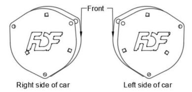
To correct camber and caster the strut spacers are designed to move the strut inward towards the engine, and back towards the rear of the car
