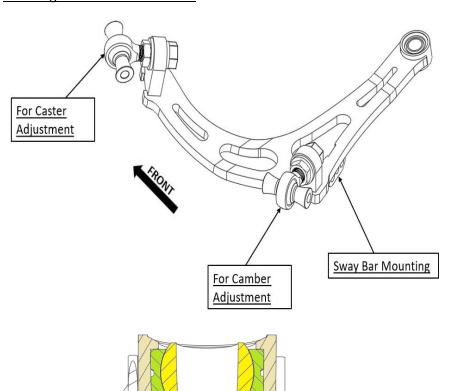
FDF Mega Mantis Lower Control Arm for BMW E90/E91/E92 is different for Left-hand and Right-hand side of the car. The Lower Control Arm shown in the image is for Right-hand side of the car.
