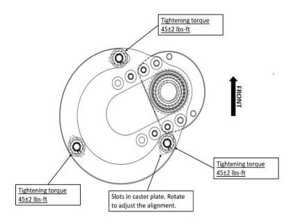
FDF Mega Mantis Caster plates for BMW E90/E91/E92 are different for Left-hand and Right-hand side of the car. The caster plate shown in the image is for Right-hand side of the car.
