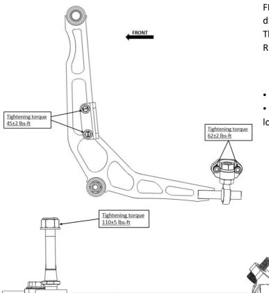
FDF Mega Mantis Lower Control Arm for BMW E46 is different for Left-hand and Right-hand side of the car. The Lower Control Arm shown in the image is for Right-hand side of the car.
