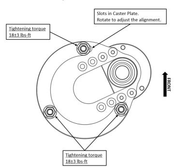
FDF Mega Mantis Caster plates for BMW E46 are different for Left-hand and Right-hand side of the car. The caster plate shown in the image is for Right-hand side of the car.
