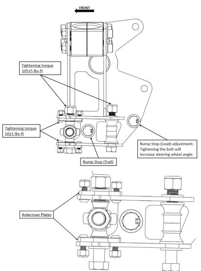
FDF Mega Mantis Knuckle for BMW E46 is different for Left-hand and Right-hand side of the car. The Knuckle shown in the image is for Right-hand side of the car.
