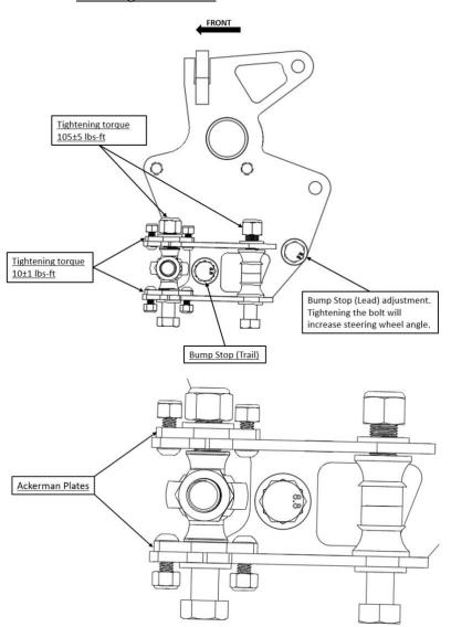
FDF Mega Mantis Knuckle for BMW E36 is different for Left-hand and Right-hand side of the car. The Knuckle shown in the image is for Right-hand side of the car.
