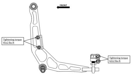
FDF Mega Mantis Lower Control Arm for BMW E36 is different for Left-hand and Right-hand side of the car. The Lower Control Arm shown in the image is for Right-hand side of the car.
