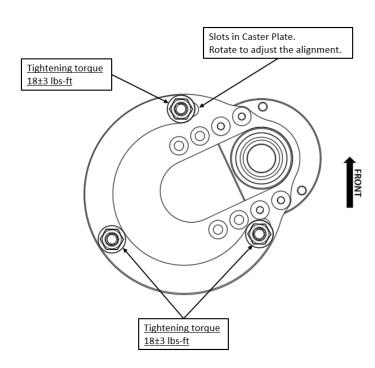
FDF Mega Mantis Caster plates for BMW E36 are different for Left-hand and Right-hand side of the car. The caster plate shown in the image is for Right-hand side of the car.
