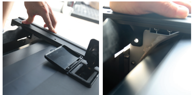
*Passenger side rail front tab installation show
