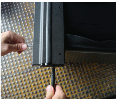
*Driver side rail front tab installation show
