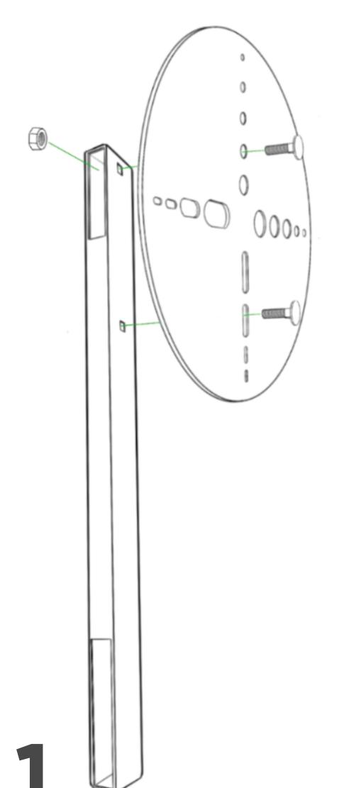
SLIDE CARRIAGE BOLT THROUGH THE PLATE AND POST. SLIDE THE NUT THROUGH POST. LIGHTLY **SCREW THE NUT ONTO** THE CARRIAGE BOLT
