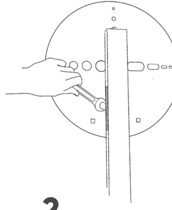
TURN THE PLATE FLAT ON THE GROUND AND TIGHTEN THE LOWER **CARRIAGE BOLT NUT** FIRST.
