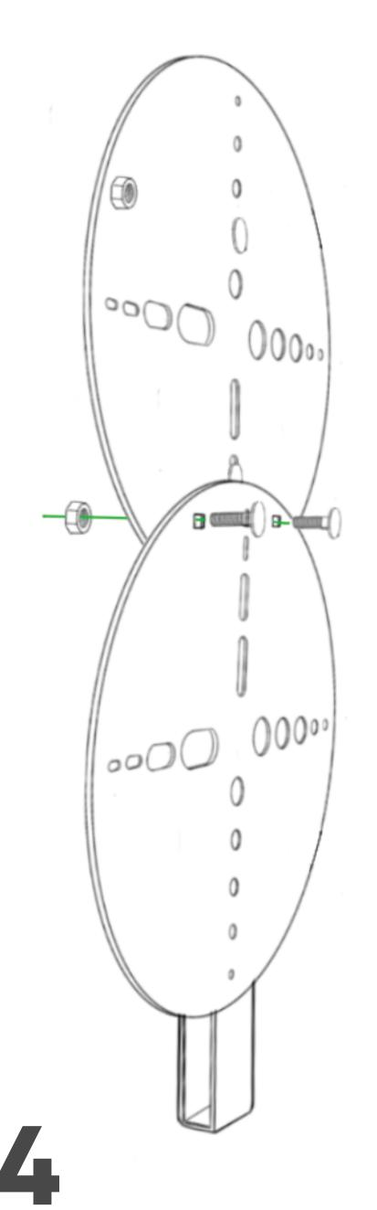
MATCH UP THE SQUARE HOLES, SLIDE THE **CARRIAGE BOLTS** THOUGH THE SQUARE HOLES AND TIGHTEN THE **NUTS FROM BEHIND.**
