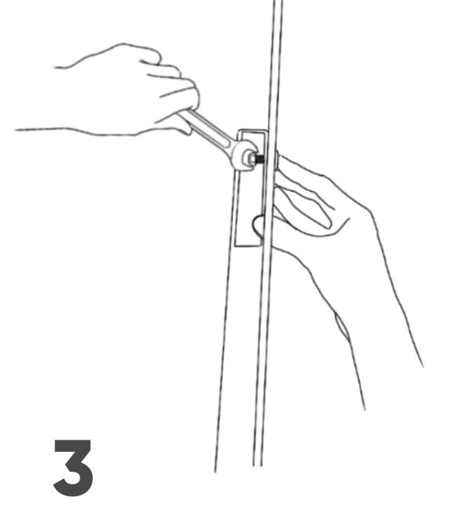
TURN THE POST ON ITS SIDE, PRESS ON THE **HEAD OF THE CARRAIGE BOLT AND TIGHTEN THE** NUT.
