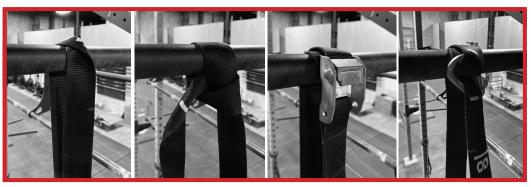
Only strap should be resting flush on anchoring point
