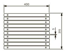
Determine which spacing you want to use. We provide a template for 5 and for 15 mm between the strips (0.2" and 0.6") for a total height of 405 or 315 mm (15.9" and 12.4") respectively.
