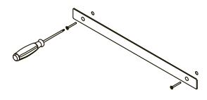
Start with the top strip and mark the holes using a spirit level. Drill holes in the wall at the marked spots and insert the wall plugs. Fasten the screws using a torx (TX-10) screwdriver.
