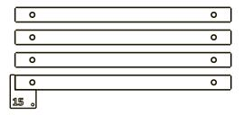
Position the spacing template at the bottom corner of the strip. Using the template, mark the location of the holes on both sides of the strip.
