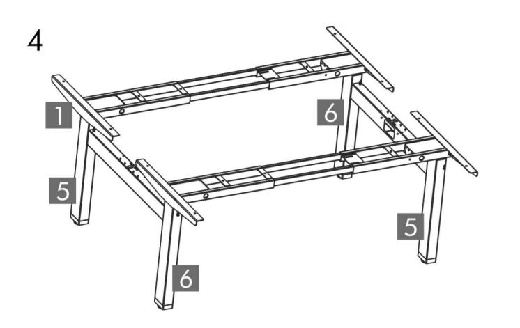
Slide the Side Brackets into thr Frames. Using eight(8) M6\*14 Machine Screws to fix the Side Brackets and Frames.
