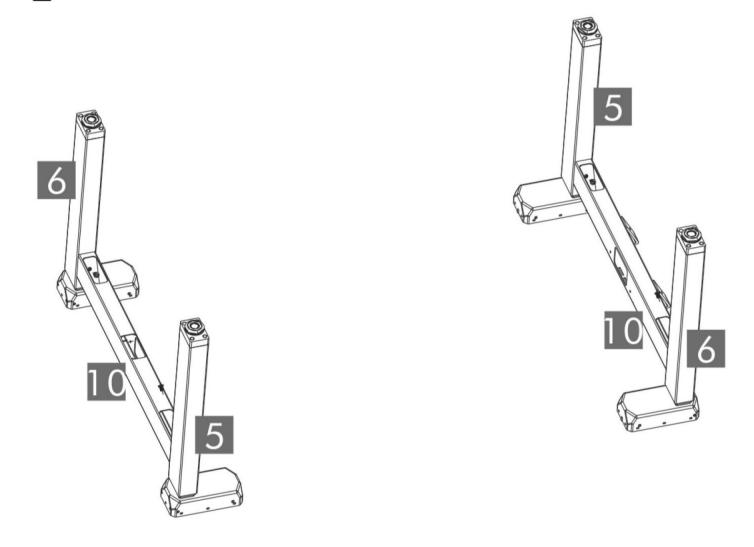
Using the supplied Allen Wrench, insert four (4) M8\*12 Machine Screws to fix the beams and legs as below picture shows.
