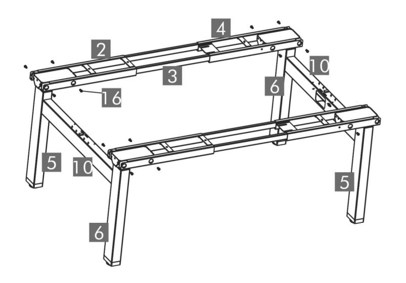
Using Sixteen(16) M6\*10 Machine Screws to fix the Frames and Legs.Put the Center Rails into Frames as below picture shows.
