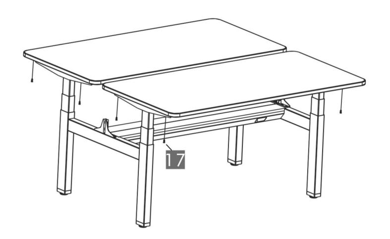
Using fourteen (14) ST5\*20 Wood Screws to fix the Table Desks with the Frames.
