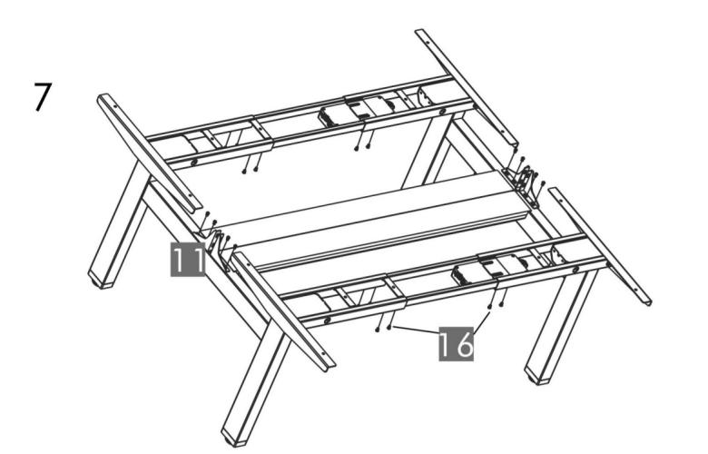
Using twenty four(24) M6\*10 Machine Screws to fix the Center Rails with Frames and Screen Holder.
