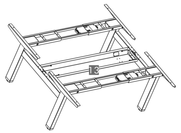
Insert four(4) M6\*10 Machine Screws into the holes of beams, assemble the Cable Tray as below picture shows.
