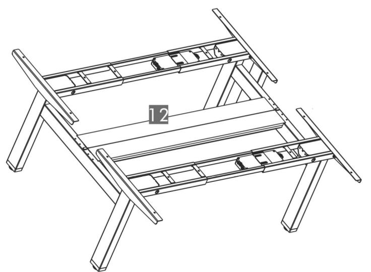
Put the Cable Tray Cover on the top of Cable Tray as below picture shows.
