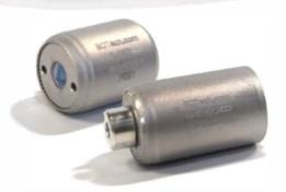
EOT's TORNOS Compact optical isolators are designed for wideranging end applications where optical feedback can adversely affect laser performance. TORNOS Compact isolators provide high transmission in the forward direction while strongly attenuating light traveling in the reverse direction, protecting lasers from the deleterious effects of back reflections.
