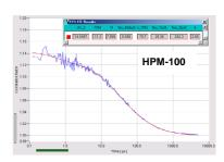
Left: Autocorrelation of continuous light signal of 10 kHz count rate, conventional GaAsP PMT. Middle: Autocorrelation of continuous light signal of 10 kHz count rate, HPM-100 module. The curve is flat down to the dead time of the TCSPC module. Right: FCS curve of fluorescein solution, HPM-100 module.
