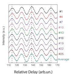
Interference patterns between the two replicas generated by the GEMINI 2D Interferometer, measured for different scan number indicated on the right. The lower one is the average of 40 scans. The measurements show an exceptional repeatibility!
