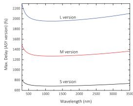
Maximum delay relative to the asymmetric (ASY) configuration achievable with the three different models (S, M and L) as a function of wavelength.
