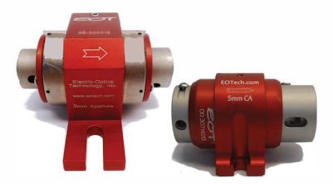
EOT's EURYS Broadband Rotators rotate the plane of polarized light 90° at 800 nm in the forward direction and 0° from 720 nm to 950 nm in the reverse direction while maintaining the light's linear polarization. When placed between crossed polarizers, a broadband Faraday rotator becomes a broadband optical isolator.
