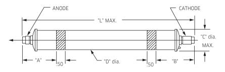
The beam exits from the anode mirror on all tubes except the 1018, 098-2 and 098-3.
